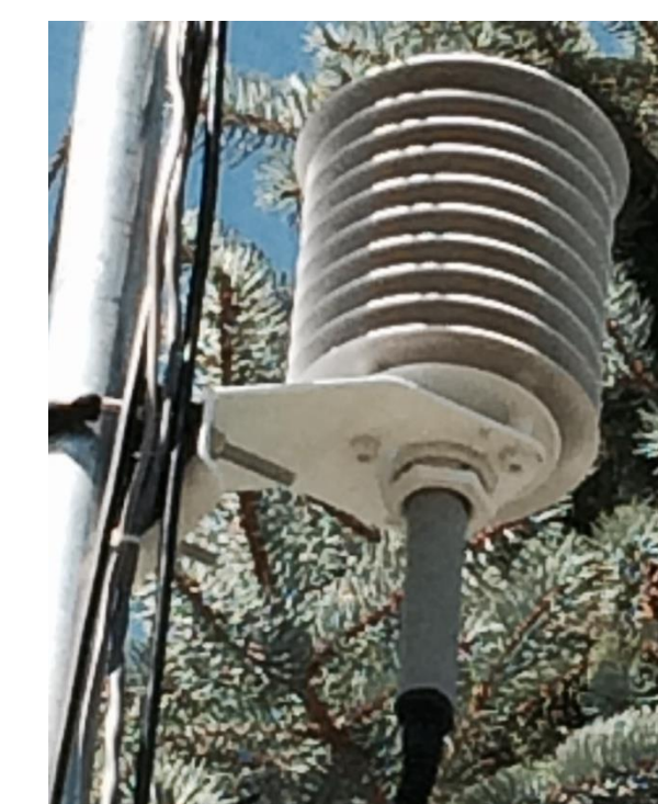
HMP45 (air temperature & relative humidity)
